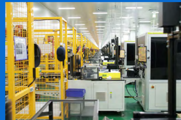
◦ Our automatic sorting and production line of monocrystalline silicon wafers
